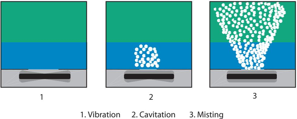
Historically, ultrasound generation of aerosol was not used often in industry because of low volume of produced aerosol. But this method has advantages such as low dispersion of produced aerosol particles and continuously adjustable volume of aerosol production.
